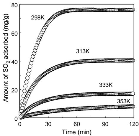
Figure 1. Effects of adsorption temperature on the amount of SO<sub>2</sub> adsorbed for static adsorption.
