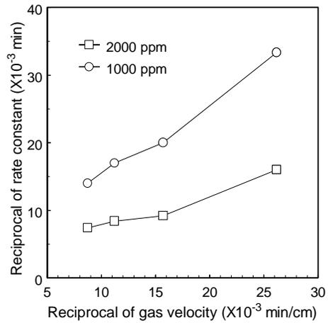
Figure 4. A plot of the reciprocal of rate constant versus the reciprocal of gas velocity for different inlet concentrations.
