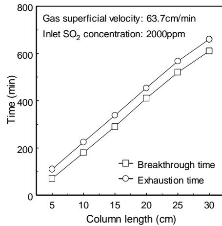
Figure 2. Effects of column length on the characteristic parameters for dynamic adsorption.
