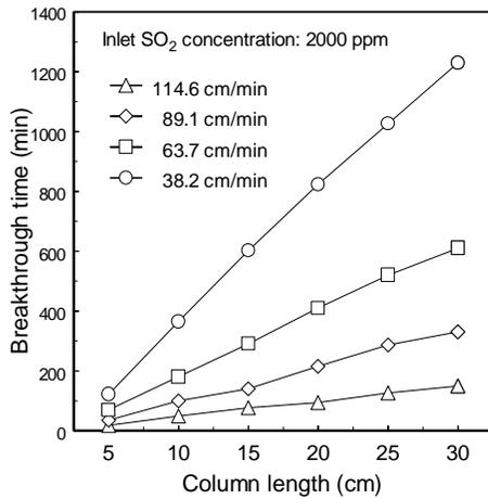
Figure 3. A plot of breakthrough time versus bed length for the fixed bed operating at various SO<sub>2</sub> superficial velocities.
