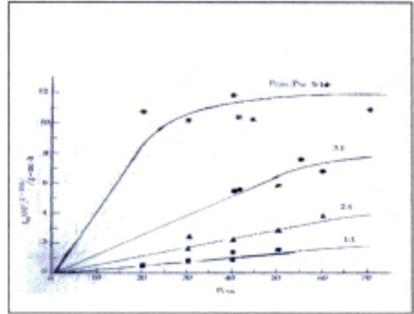
Fig 3. Deposition rate vs. partial pressure of hydrogen
