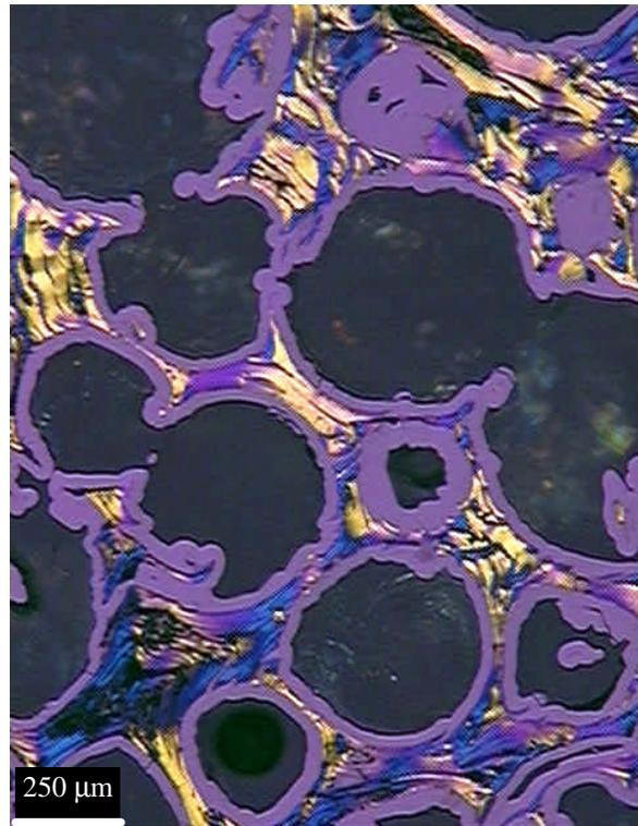
Figure 1. Optical Micrographs of carbon foam before and after coating with silicon carbide.
