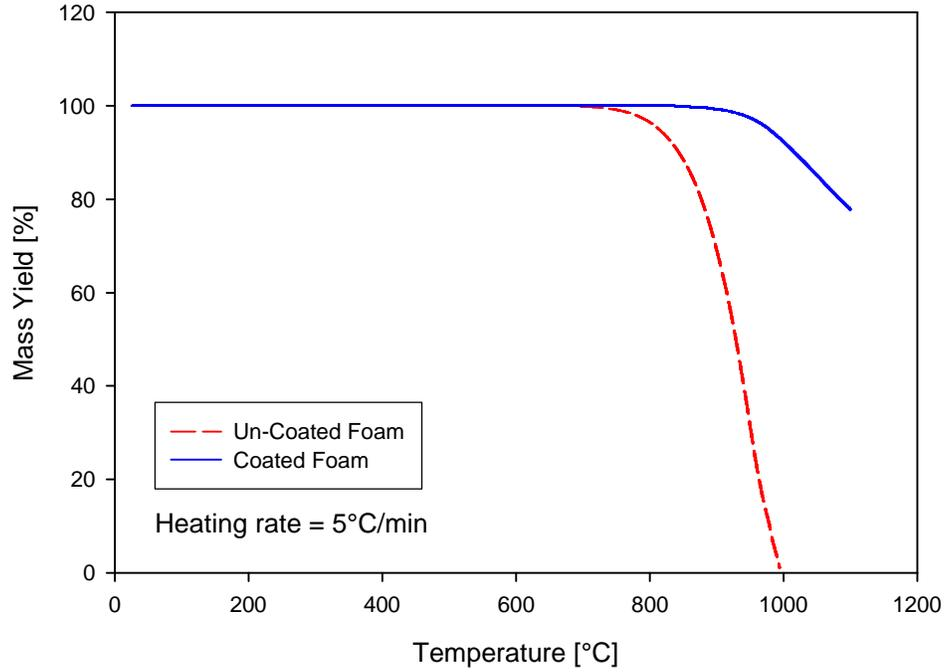
Figure 4. TGA plot of the uncoated and coated foams in air and temperatures up to 1100C.
