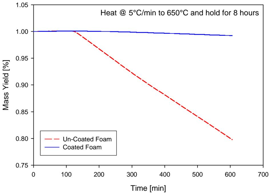
Figure 5. TGA plot of the uncoated and coated foams held in air at 650C for 8 hours.
