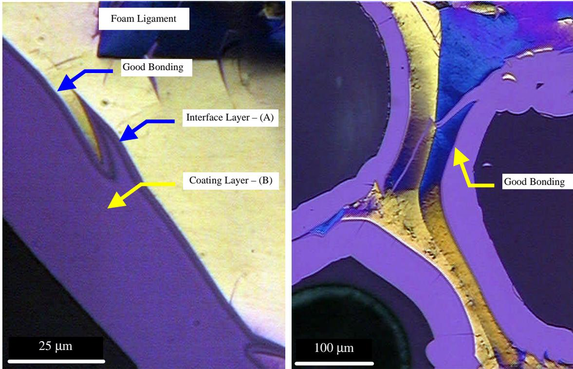
Figure 2. High magnification images of the interface between the foam and the coating illustrating a 3 layer coating.
