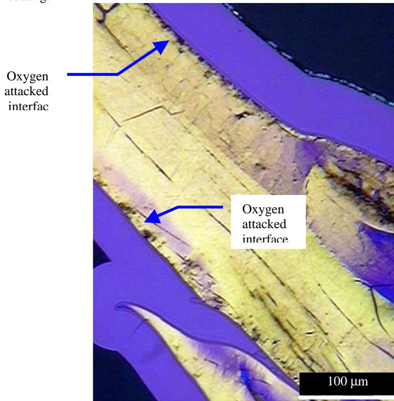
Figure 3. High magnification image of interface after oxidation in air at 650°C for 8 hours.
