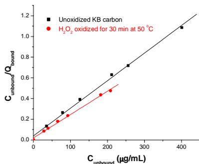
Figure 1. Langmuir isotherms of doxorubicin binding onto activated carbons
