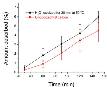
Figure 2. Desorption of the adsorbed doxorubicin from initial activated carbons
