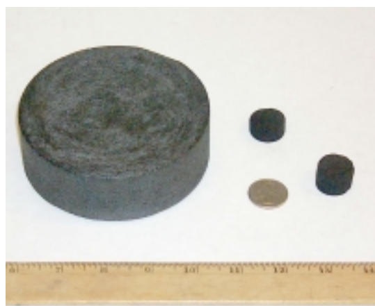
Figure 2. Gas storage monolith and test specimens
