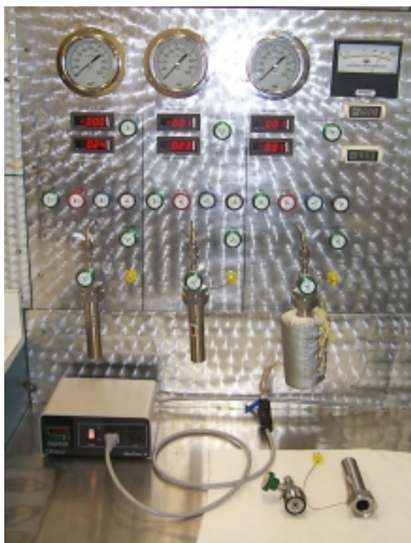
Figure 3. Methane adsorption test apparatus
