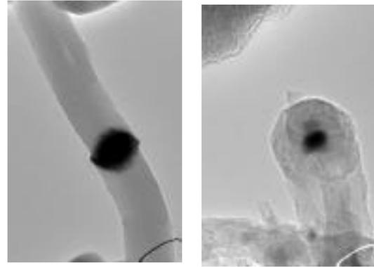
Figure1. TEM images for (a) “Herringbone” and (b) “tubular” carbon fibers.
