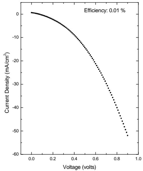
Fig.4 Illuminated J-V curve of phosphorous ion implanted C<sub>60</sub> film /p-Si
