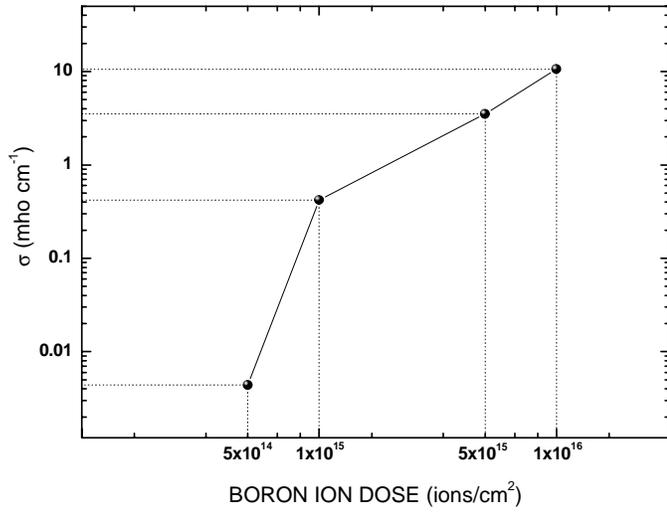
Fig. 1 Conductivity vs boron ion dose
