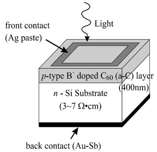
Fig 2 Schematic figure of the cell
