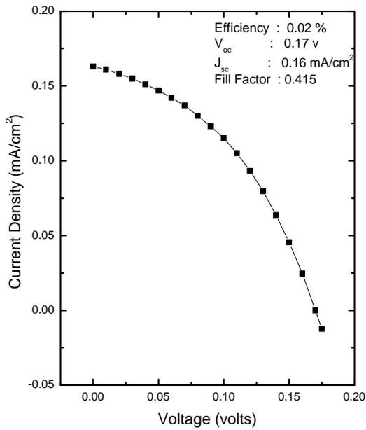
Fig. 3 Illuminated J-V curve of boron ion implanted C<sub>60</sub> film/n-Si
