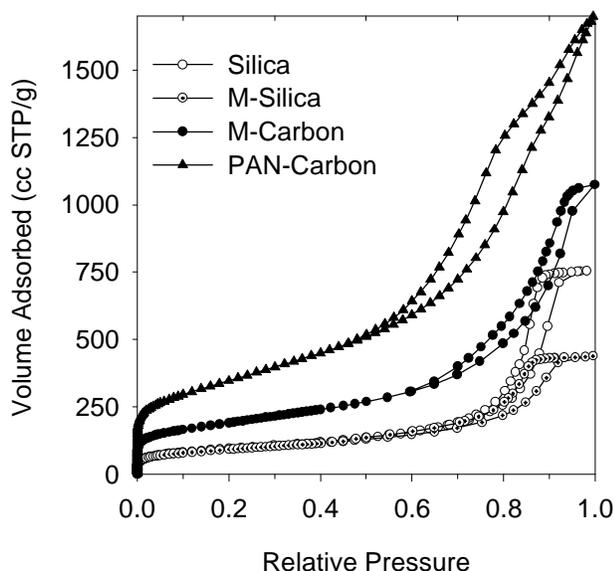
**Figure 1.** Nitrogen adsorption isotherms for the initial silica, the mesophase pitch-silica hybrid (M-Silica) and the mesoporous carbons obtained by dissolving silica from the hybrid samples at  $-196\text{ }^{\circ}\text{C}$ .
