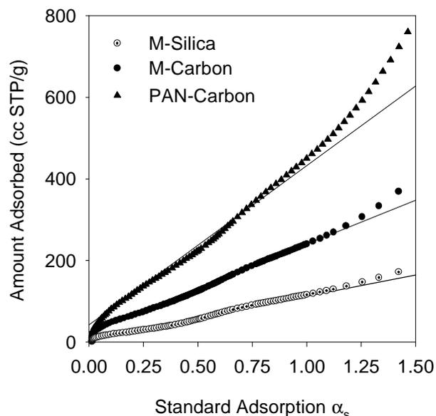
**Figure 3.** The  $\alpha_s$ -plots for the samples studied prepared by using standard adsorption data reported in [6].
