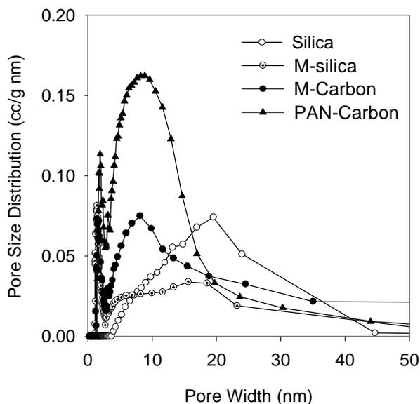
**Figure 2.** Pore size distributions for the initial silica, the mesophase pitch-silica hybrid (M-Silica) and the mesoporous carbons obtained by dissolving silica from the hybrid samples calculated according to the BJH method from nitrogen adsorption isotherms shown in Figure 1.
