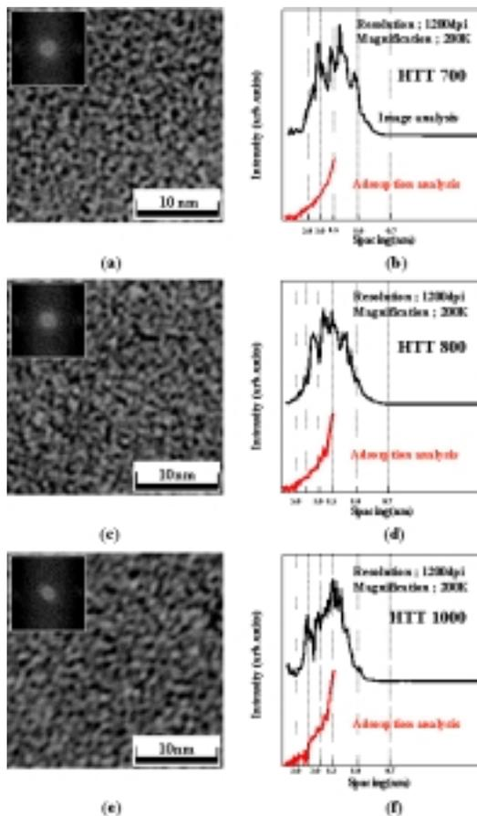
corresponding pore size distributions of PVDC-base carbon samples, VESC, in comparison to the PSD
