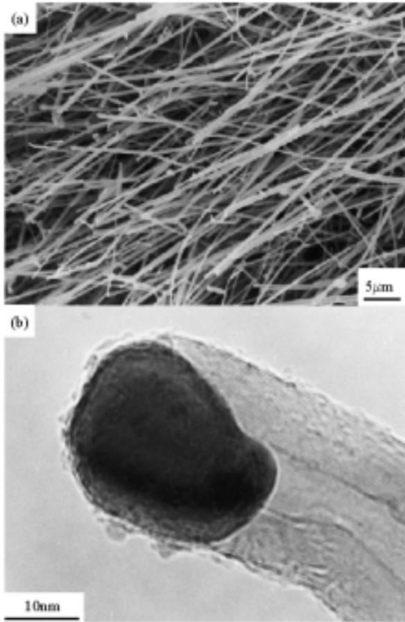
Figure 2. (a) FE-SEM of VGCFs and (b) TEM images showing early stage of growth in the floating reactant method.
