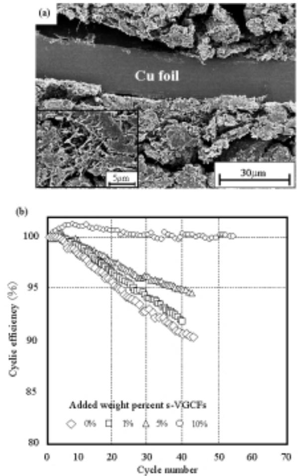
Figure 4. (a) Practical anode cell containing thin VGCFs, (b) cyclic characteristic of synthetic graphite as a function of added weight percent of thin VGCFs.
