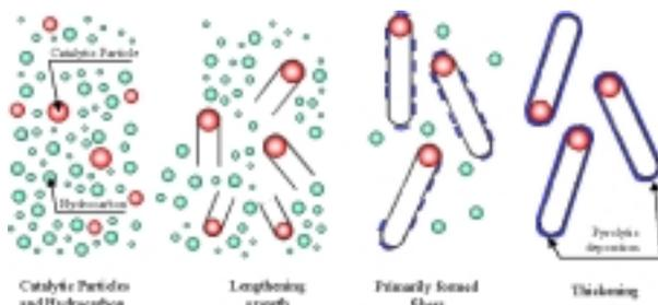
Figure 3. Suggested growth mechanism of thin VGCFs in floating reactant method
