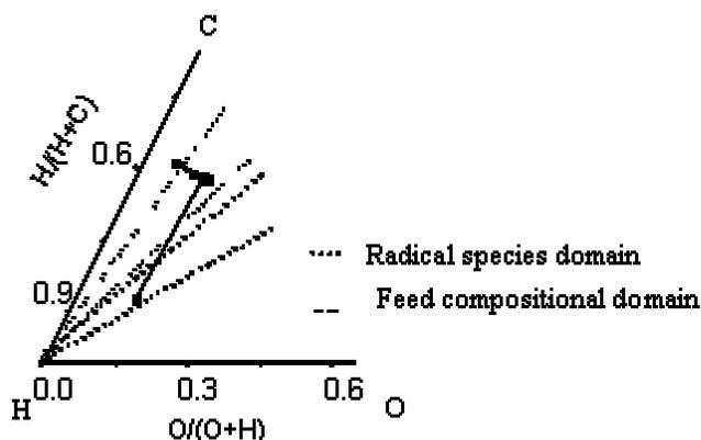
Figure 2. The effect of increasing boron concentration on the resulting radical species composition for feed gas composition located within diamond deposition domain.
