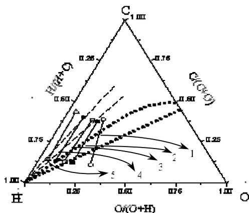
Figure 1. The position of data points with respect to feed gas composition and radical species compositions. The lens shaped region is given by feed gas compositions<sup>2</sup> and the upper region is described by radical species composition<sup>3</sup>.
