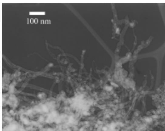
Fig. 4. TEM micrograph of MWNTs grown on Tb:Fe-coated Si substrate at 700 °C for 120 mins.
