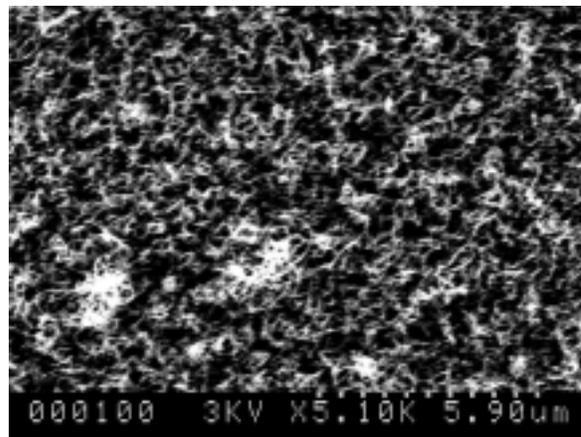
Fig. 3. SEM micrograph of MWNTs grown on Fe-coated Si substrate at 700 °C for 120 mins.
