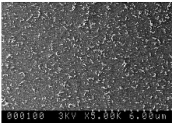
Fig. 2. SEM micrograph of MWNTs grown on Tb:Fe-coated Si substrate at 700 °C for 60 mins.
