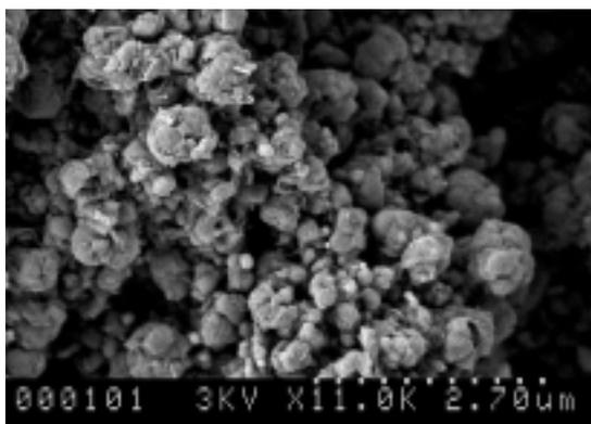
Fig. 5. SEM micrograph of graphitic particles formed on Cu-coated alumina substrate at 700 °C for 120 mins. Decomposition of a ferrocene-xylene mixture at 700 °C over a Cu-coated alumina substrate produced cauliflower-
