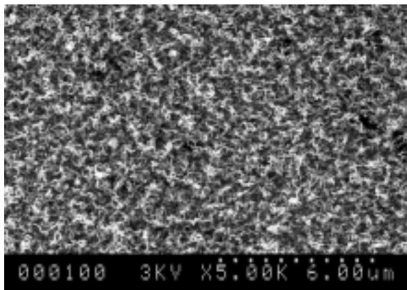
Fig. 1. SEM micrograph of MWNTs grown on Tb:Fe-coated Si substrate at 700 °C for 120 mins.
