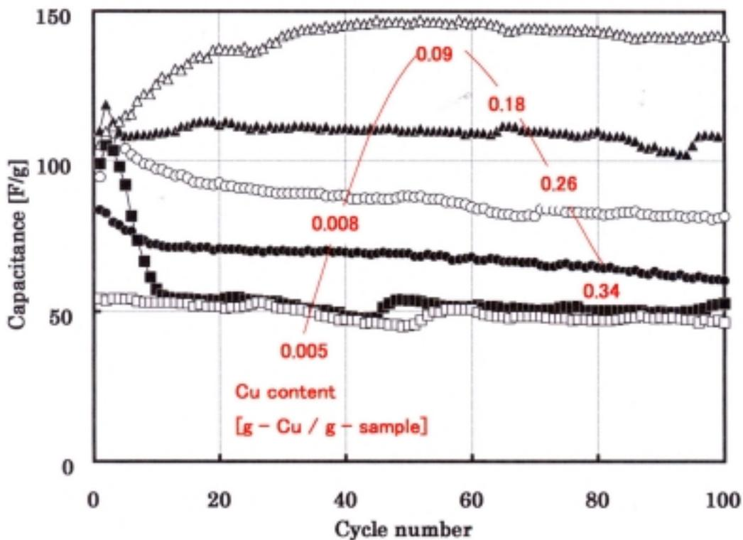
Fig. 3 The capacitance change with cyclic number of various Cu - content carbon electrode prepared by C467-Cu<sup>2+</sup>.
