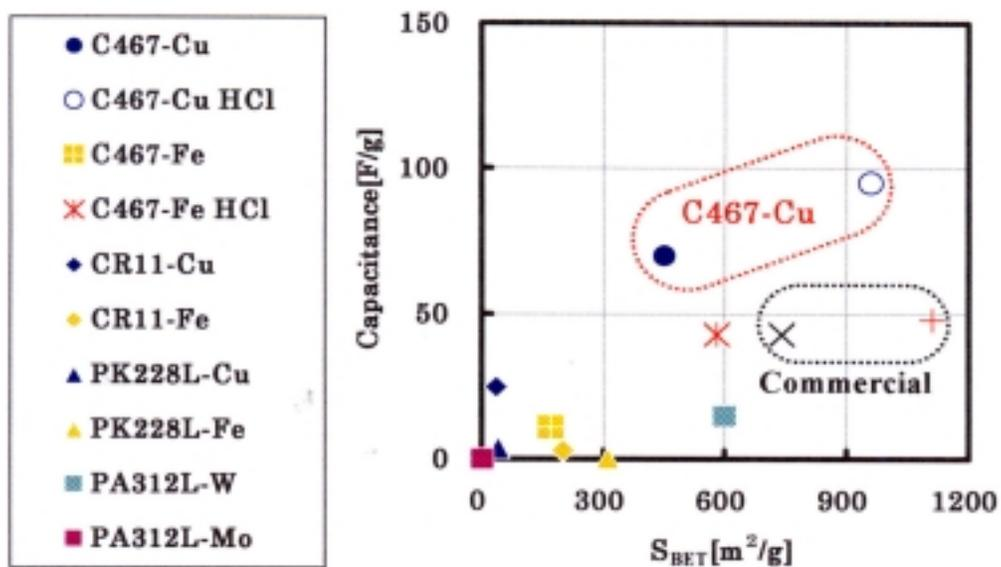
Fig. 2 The relation of the capacitance of EDLC and  $S_{BET}$ .
