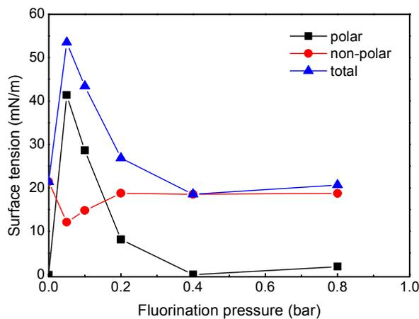
Fig. 2. Surface tension of fluorinated carbon fiber as a function of fluorination pressure (F<sub>2</sub>/O<sub>2</sub>=1, fluorination time = 30min).
