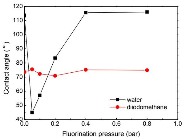
Fig. 1. Contact angle of fluorinated carbon fiber as a function of fluorination pressure (F<sub>2</sub>/O<sub>2</sub>=1, fluorination time = 30min).
