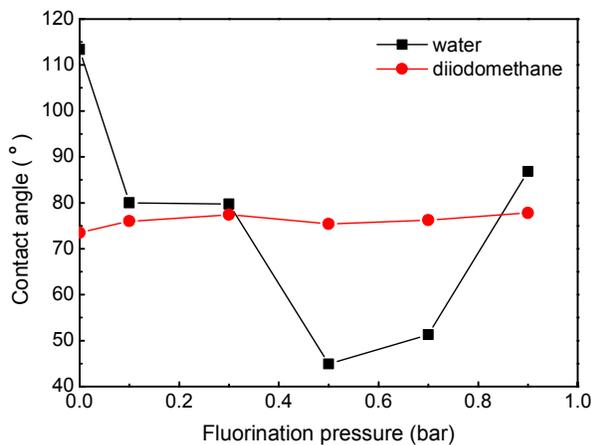
Fig. 3. Contact angle of fluorinated carbon fiber as a function of O<sub>2</sub> partial pressure (fluorination pressure = 0.05bar, fluorination time = 30min).
