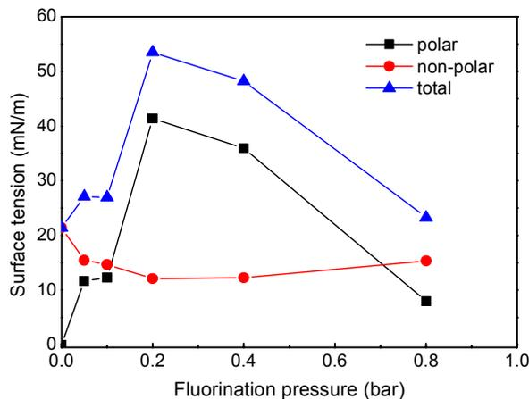
Fig. 4. Surface tension fluorinated carbon fiber as a function of O<sub>2</sub> partial pressure (fluorination pressure = 0.05bar, fluorination time = 30min).
