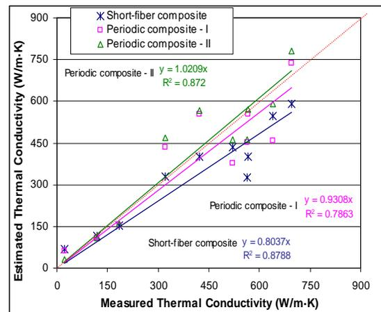
Figure 3. Measured versus estimated values of thermal conductivity for ribbon and round fibers.
