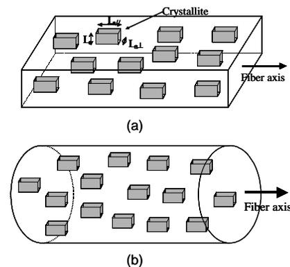
Figure 1. Schematic of a (a) ribbon fiber and (b) round fibers visualized as an aligned short-fiber composite.
