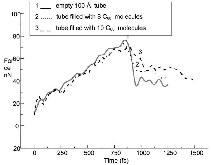
Fig.2 Force curves for the compression of a 100 Å long carbon nanotube filled with various densities of C<sub>60</sub>.
