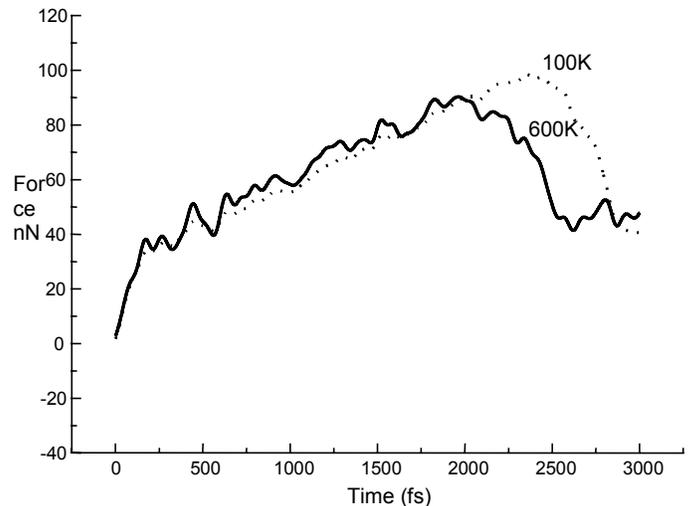
Fig.4 Force curves for the compression of a 200 Å long carbon nanotube filled with Ne at various temperatures
