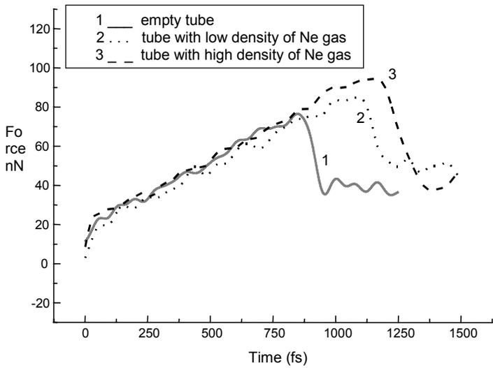
Fig.1 Force curves for the compression of a 100 Å long carbon nanotube filled with various densities of Ne.
