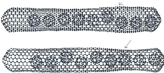
Fig.3 Side and top views of nanotube compression. The arrow indicates the moment before buckling.
