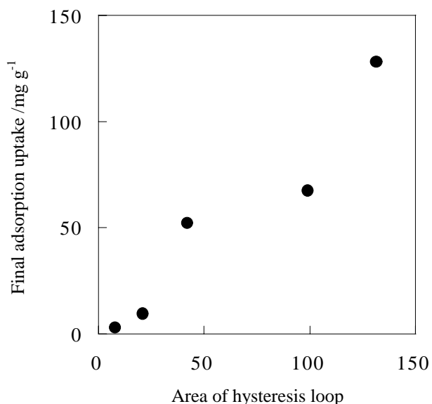
Figure 6. Relationship between the area of water adsorption hysteresis loop and the final adsorption uptake on the water-adsorbed microporous carbons at 303 K.
