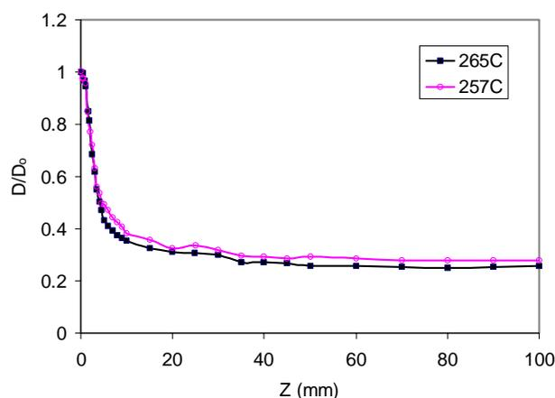
Figure 4. Effect of spinning temperature on the fiber diameter profiles. DDR was 12.1.
