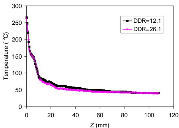
Figure 1. Effect of DDR on the fiber surface temperature profiles. Spinning temperature was 265 °C.
