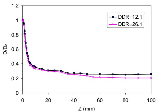
Figure 3. Effect of DDR on the fiber diameter profiles. Spinning temperature was 265 °C.
