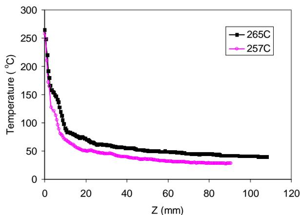
Figure 2. Effect of spinning temperature on the fiber surface temperature profiles. DDR was 12.1.
