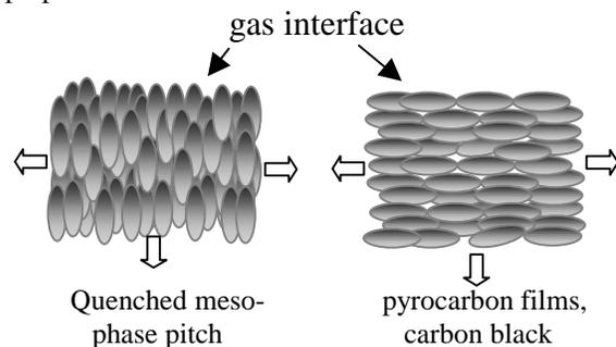
**Figure 2.** Structures observed at the gas interface for quenched mesophase pitch and selected carbon materials. These structures indicate a dominant face-to-face assembly process for pitch (left) and edge-to-edge assembly process for pyrocarbon and carbon black.
