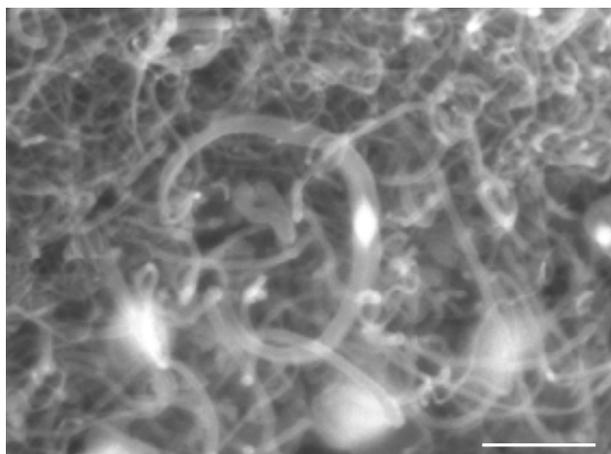
Fig. 1. SEM micrograph of carbon nanofibres grown by thermal CVD process using acetylene. Large bi-directional carbon nanofibre with diamond shape catalyst particle can be seen in the center.
