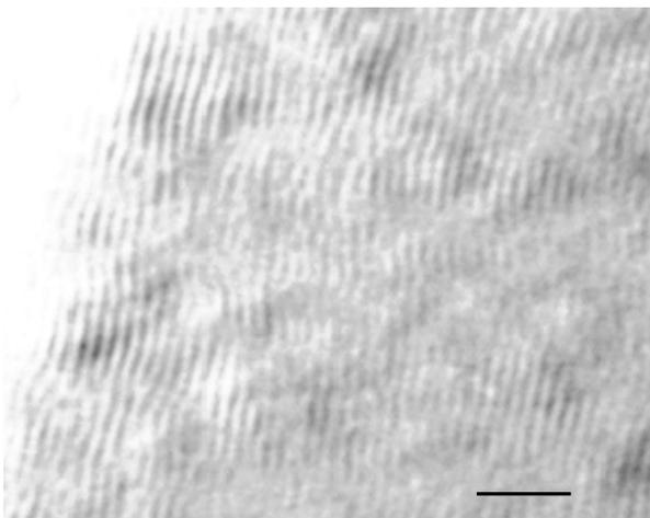
Fig. 3. Enlarged part of the carbon nanofibre showing carbon lattice fringe images almost parallel to the surface of the nanofibre.
