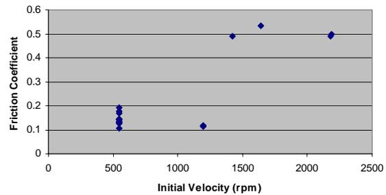
Figure 6. Average friction coefficient of needled felt C/C (type A) after HHT under variety of initial stop velocities. Stops 56-73 of data shown in Fig 5.
