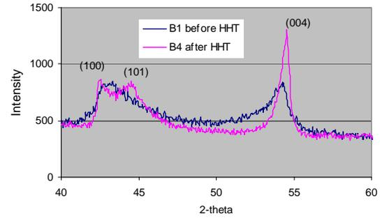
Figure 2. XRD pattern for needled felt C/C before and after HHT.
