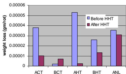
Figure 9. Wear rates for dynamometer testing of needled felts before and after HHT. Specimens A and B tested under Cold Taxi (ACT, BCT), Hot Taxi (AHT, BHT) and Normal Landing (ANL) conditions.
