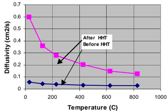
Figure 3. Through-thickness thermal diffusivity of needled felt C/C ( $\sim 15\%$  z-fiber) before and after HHT.
