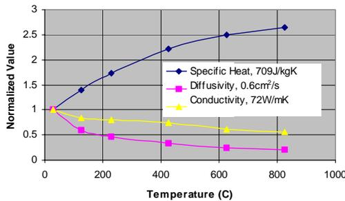
Figure 4. Through-thickness thermal properties of needled felt C/C (~15% z-fiber) after HHT. Room temperature values were used to normalize data as shown.
