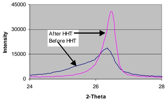
Figure 1. XRD pattern for needled felt C/C before and after HHT.
