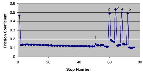
Figure 5. Average friction coefficient of needled felt C/C (type A) after HHT under variety of stop conditions as indicated in the text . RH = 54%..
