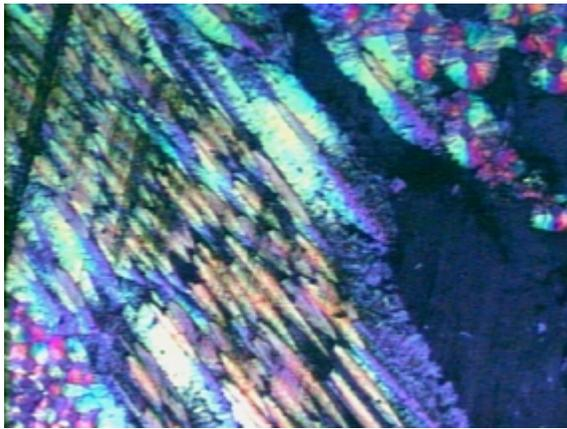
Figure 7. Friction surface after dry cold taxi stops (above transition) showing polished surface with minimal friction film present.
