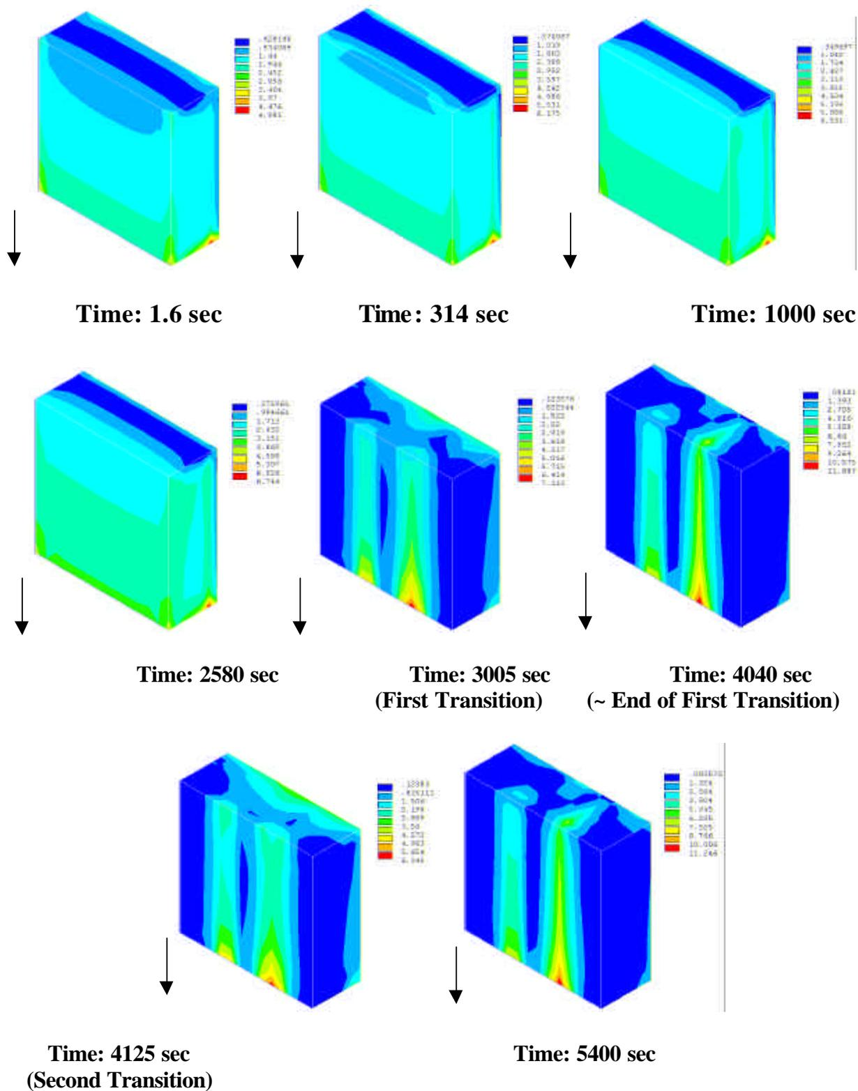
**Figure10.** Cracks generation in the samples of various testing conditions. The arrows indicate rubbing directions.
