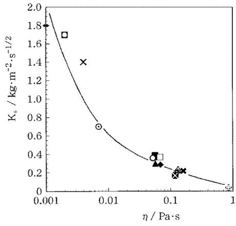
Fig. 4 Dependence of sorptivity  $K_s$  on viscosity  $\eta$ .
