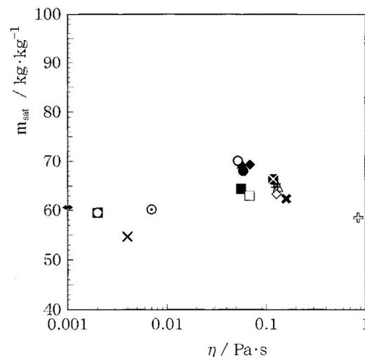
Fig. 3 Saturated sorption capacity  $m_{sat}$  against viscosity  $\eta$  of oils
