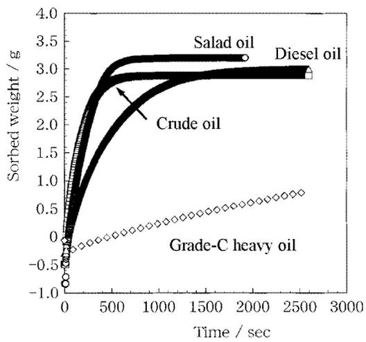
Fig. 2 Sorption curves for the oils with different viscosity
