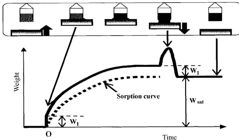
Fig. 1 Schematic illustration of wicking method.
