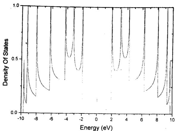
**Figure 3.** Density of states versus energy for a (5,5) armchair metallic tube
