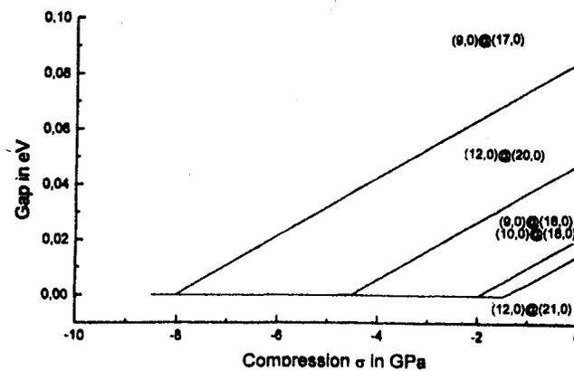
**Figure 4.** Semiconductor-metal transitions for selected double-walled carbon nanotubes
