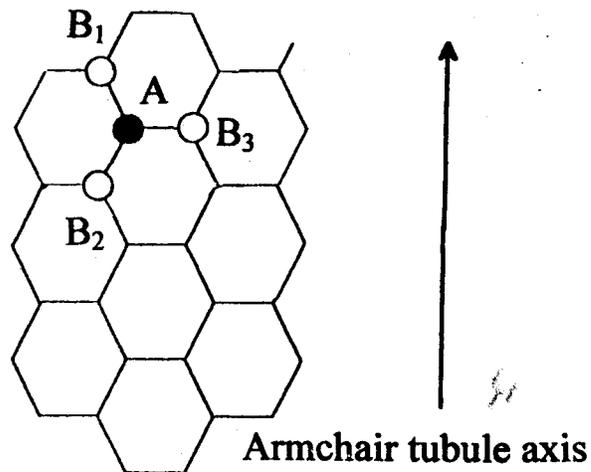
**Figure 2.** Armchair single-walled carbon nanotube
