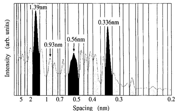
Figure 4. Judgment of the degree of the peaks obtained by integration of the power spectrum of Fig.3 by fuzzy reasoning.
