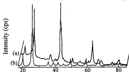
**Figure 3.** XRD patterns of (a) the reaction products and (b) reactant SiO<sub>2</sub>. (a) 30 kV, 25 mA; (b) 25 kV, 5 mA.
