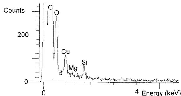
**Figure 2.** EDS spectra of one straight whisker in the reaction products. (Cu signal occurs from the Cu grid.)
