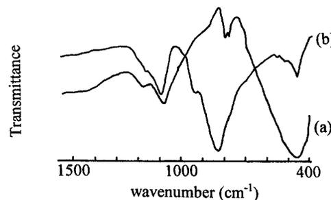
**Figure 4.** FT-IR spectra of (a) the reaction products and (b) the commercial SiC.
