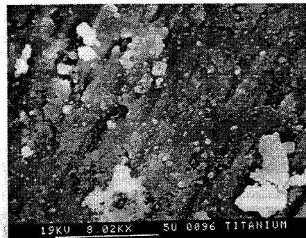
Figure 3. Deposit morphology on Ti.
