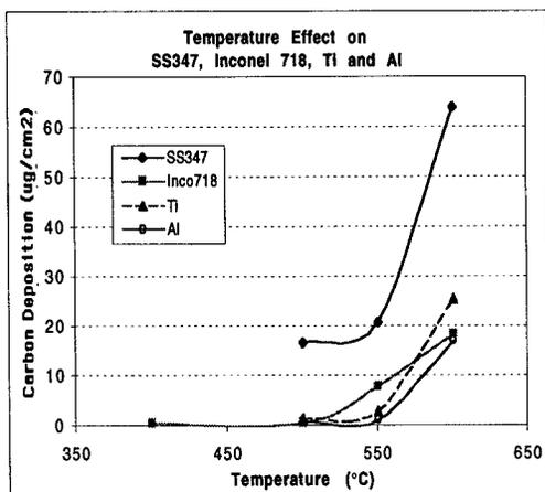
Figure 1. Effect of temperature on deposition
