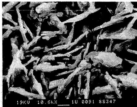
Figure 2. Deposit morphology on SS347.
