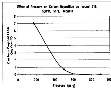
Figure 5. Effect of pressure on deposition.
