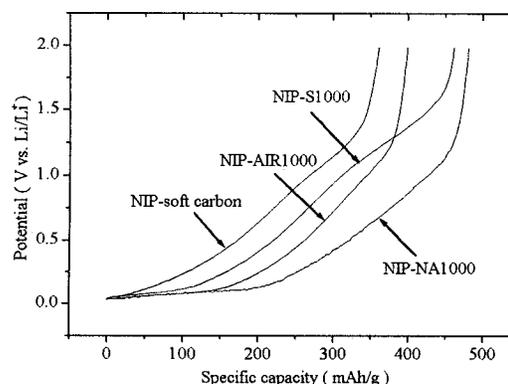
Figure 2. Discharge profiles of hard carbons prepared from the naphthalene pitch by different cross-linking methods.
