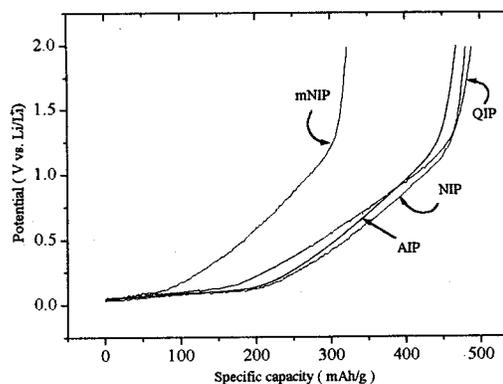
Figure 3. Discharge profiles of hard carbons prepared from oxidized synthetic isotropic pitches with nitric acid treatment.
