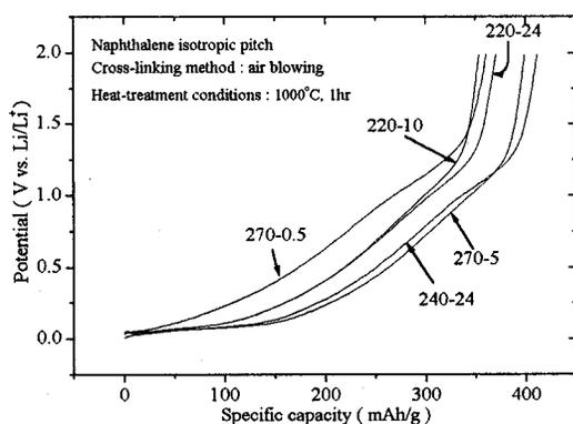
Figure 1. Discharge potential profiles of hard carbons prepared from naphthalene isotropic pitch with air blowing under different conditions.
