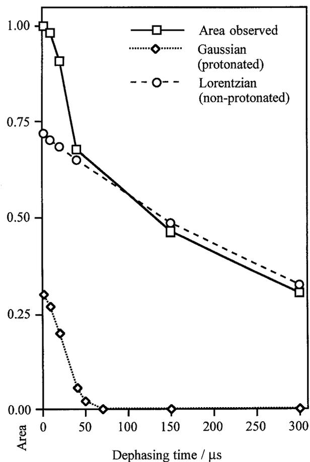
**Figure 2.** Variation in area observed for the aromatic peak with respect to the dephasing time for the quinoline insoluble fraction of coal tar pitch D.
