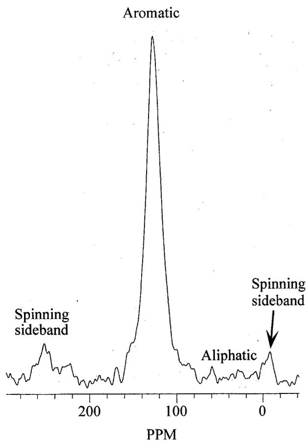
**Figure 1.** Solid state  $^{13}\text{C}$  NMR spectrum of the whole binder pitch A, using the quantitative single pulse excitation technique.
