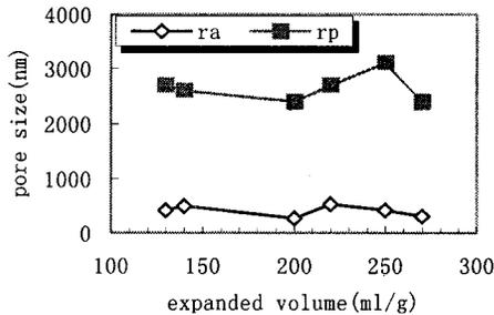
Fig.2 The pore size of EG with different exfoliation volume
