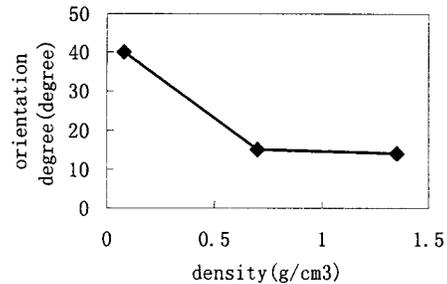
Fig.4 The relationship between orientation degree of (002) plane and density of FGS
