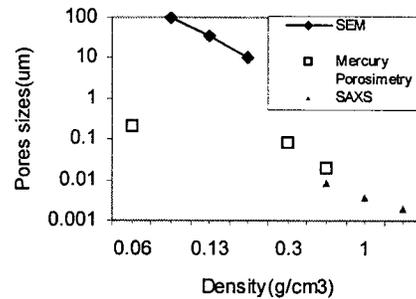
Fig.3 Mean pore diameter variance of FG with its density
