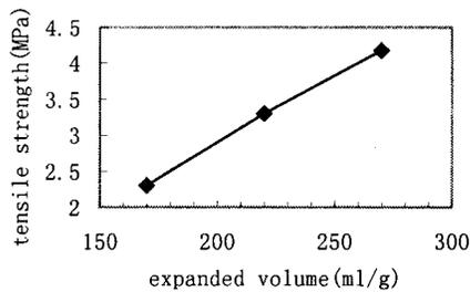
Fig.1 The Effect of exfoliation volume on tensile strength ( $\rho = 0.8\text{g/cm}^3$ )
