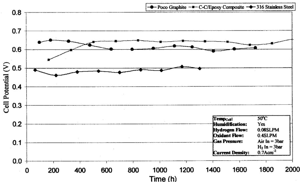
**Figure 2.** Average weekly cell potential at constant current density (0.7A/cm<sup>2</sup>)
