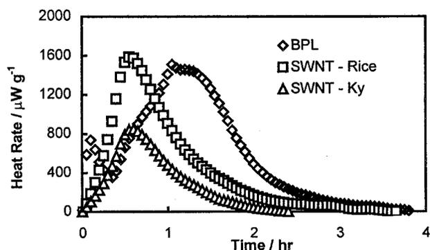
Figure 1: Calorimetry results for hydrogen adsorption.
