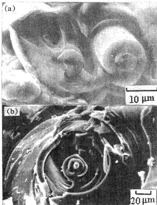
Figure 2 The laminal structure of pyrocarbon
