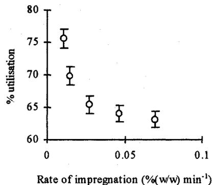
**Figure 4.** The effect of rate of impregnation on impregnant utilisation
