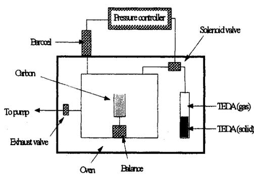
**Figure 1.** TEDA adsorption apparatus
