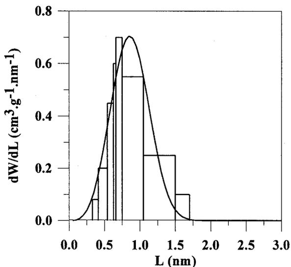
Figure 3. Pore size distribution for activated carbon EP1 (burn-off 37%) determined by CO<sub>2</sub> adsorption and immersion calorimetry.
