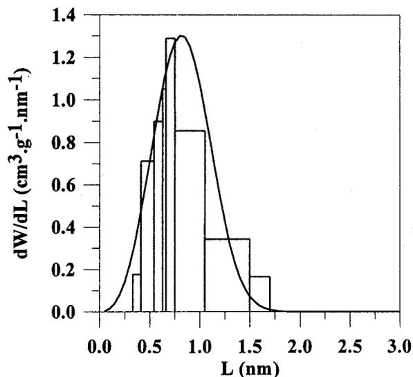
Figure 4. Pore size distribution for activated carbon EP2 (burn-off 37%) determined by CO<sub>2</sub> adsorption and immersion calorimetry.
