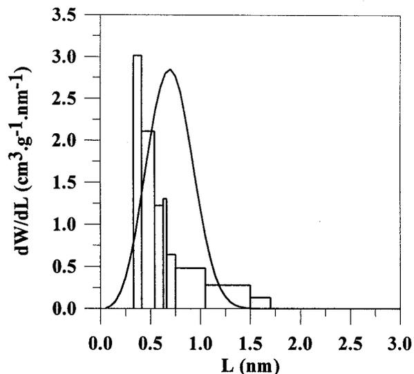
Figure 2. Pore size distribution for activated carbon EP2 (burn-off 13%) determined by CO<sub>2</sub> adsorption and immersion calorimetry.
