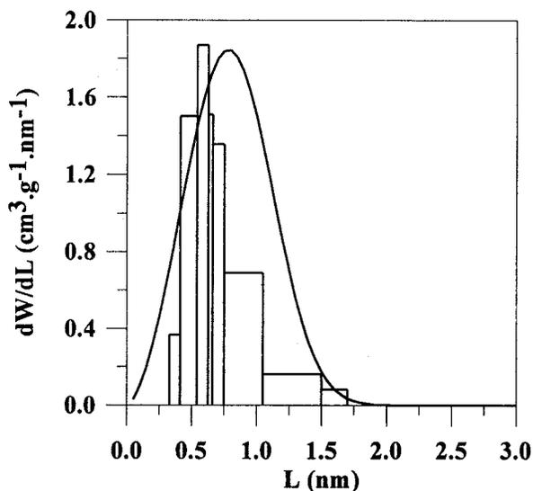
Figure 1. Pore size distribution for activated carbon EP1 (burn-off 12%) determined by CO<sub>2</sub> adsorption and immersion calorimetry.
