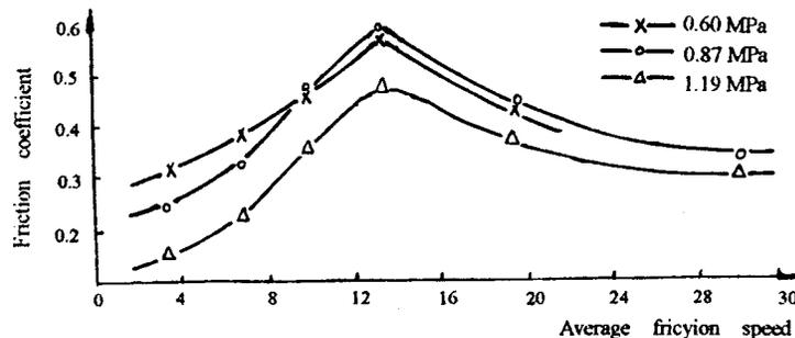
Fig.1 Variation of friction coefficient of C/C composite discs with friction speed
