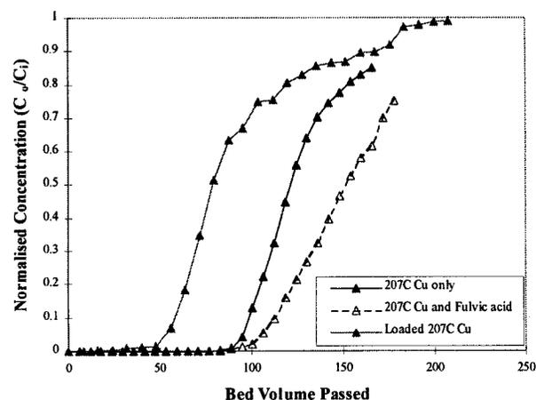
**Figure 3:** Breakthrough curves generated using Sutcliffe Speakman 207C
