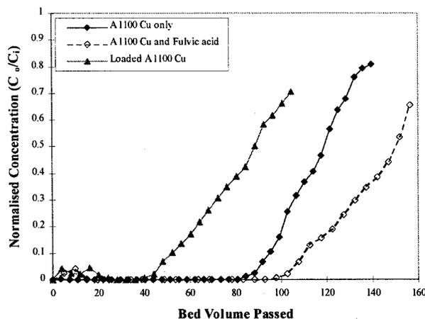
**Figure 2** Breakthrough curves generated using Westvaco A1100
