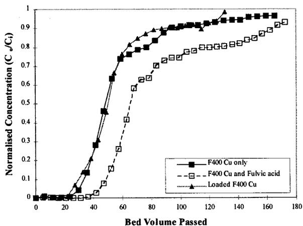
**Figure 1:** Breakthrough curves generated using Chemviron F400
