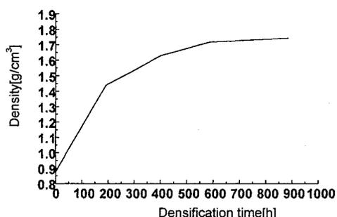
Figure 1. Relationship between material density and densification time
