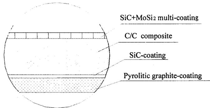
Figure 1. Schematic of the multi-coating
