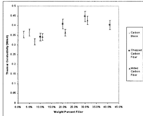
Figure 3. Through-Plane Thermal Conductivity Results versus Weight Percent filler for Nylon 6,6 Based Conductive Resins
