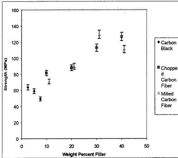
Figure 1. Tensile Strength versus Weight Percent Filler for Nylon 6,6 Based Conductive Resins
