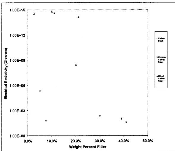
Figure 2. Electrical Resistivity (in ohm-cm) Results versus Weight Percent for Nylon 6,6 Based Conductive Resins
