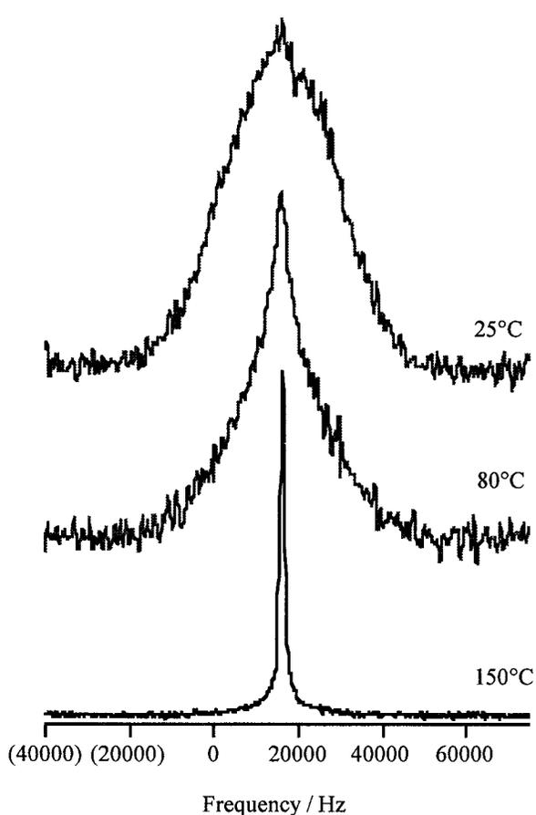
**Figure 1.** High temperature  $^1\text{H}$  NMR spectra of the binder pitch B at ambient temperature (25°C, top), 80°C (middle) and 150°C (bottom) showing the effect of softening upon the NMR signal.
