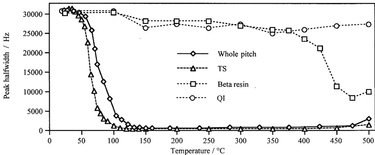
**Figure 2.** Variation in the peak half-width for binder pitch A and its TS, beta resin and QI fractions with temperature.
