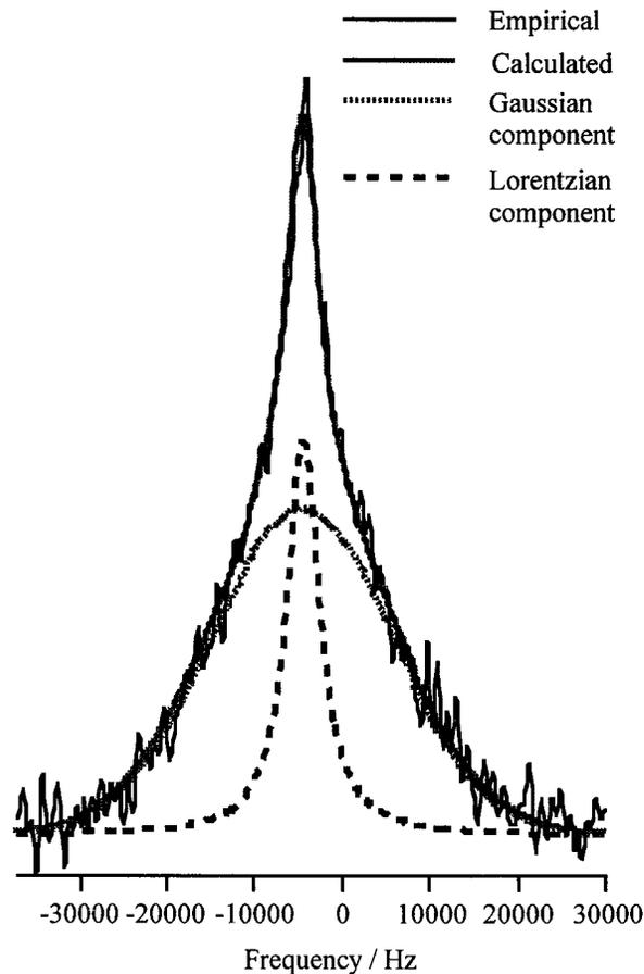
**Figure 3.** High temperature  $^1\text{H}$  NMR spectrum of the beta-resin fraction of binder pitch A at maximum fluidity at 475°C deconvoluted into its fluid or Lorentzian component, and its rigid or Gaussian component.
