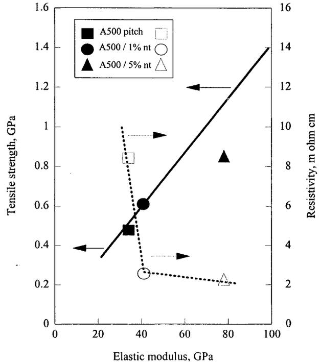
Fig. 2 Experimental values of properties of nanotube-pitch composite carbon fibers.
