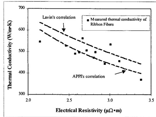
Figure 1. Values of thermal conductivity, measured with Angstrom's apparatus, versus the measured room-temperature electrical resistivity for ribbon fibers.
