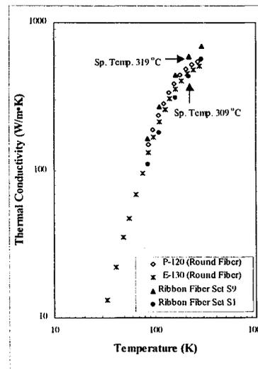
Figure 3. Temperature-dependence thermal conductivity of two sets or ribbon fibers and two types of commercial round fibers.
