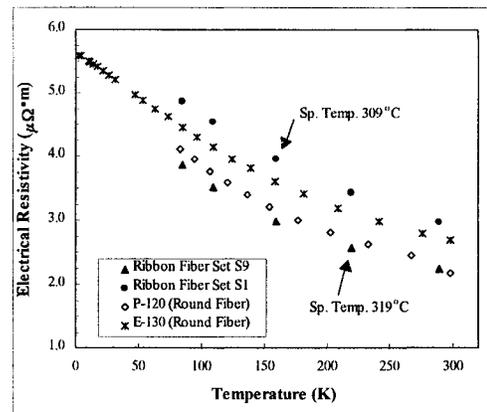
Figure 2. Temperature-dependence electrical resistivity of two sets or ribbon fibers and two types of commercial round fibers.
