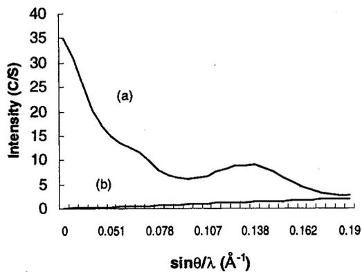
Figure 1. Diffraction pattern for graphite ground 74 hours. (a) Complete pattern. (b) Compton (incoherent) background
