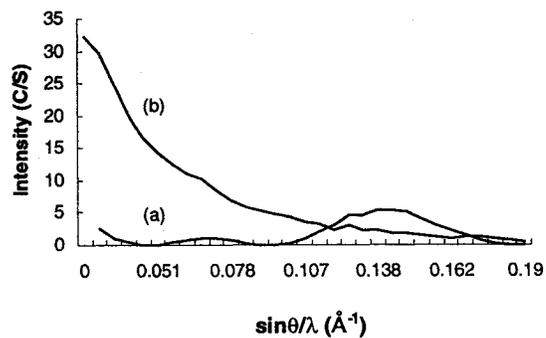
Figure 2. Components of the intensity data for C74 material. (a) Bragg diffraction. (b) Small angle scattering.
