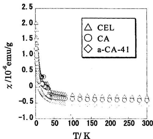
Fig.2  $\chi$ -T plots of Cellulose-based ACF (CEL), CA, and a-CA.
