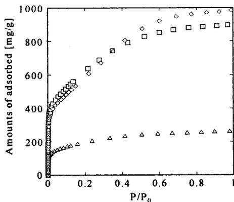
Fig.1 Adsorption isotherms of nitrogen on a-MCMB activated by KOH
