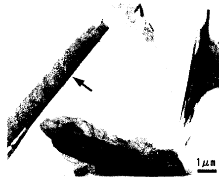
Figure. 3 TEM image of pitch C heat-treated at 2500°C. Specific morphology indicated by arrow is found among the normal phase particles.
