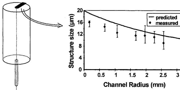
Figure 5. Observed vs. predicted transverse structure in reservoir during mesophase extrusion [4].
