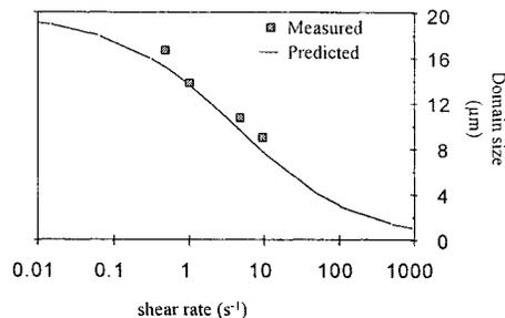
Figure 2. Comparison between predicted and measured domain size during shear flow of a mesophase [2].
