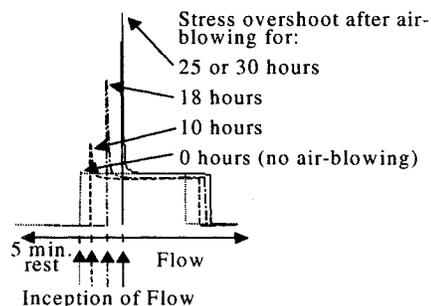
Figure 1. Stress response upon start-up of shear flow for untreated and air-blown pitches [1].
