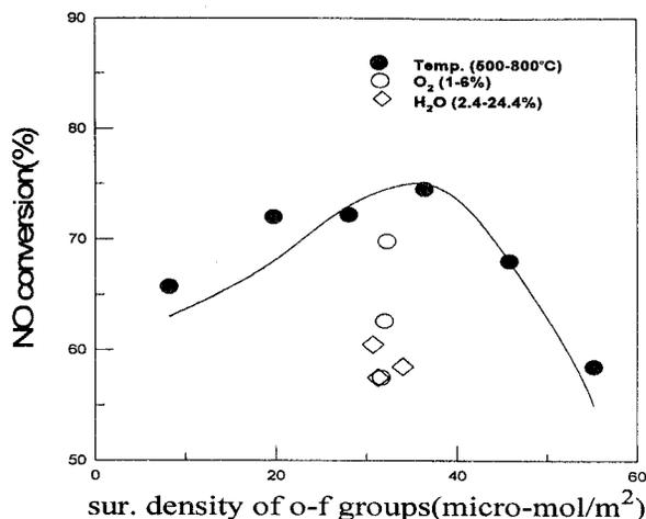
Figure 2. Relationship between the NO conversion and the density of oxygen-functional groups of activated carbons prepared under various kinds of pyrolysis conditions.
