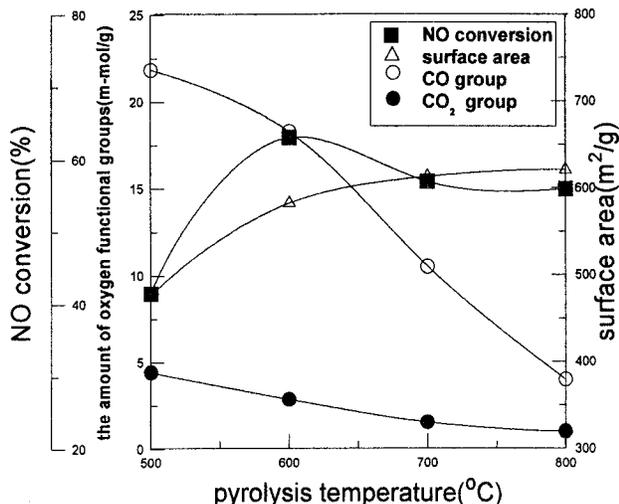
Figure 1. Effect of pyrolysis temperature on surface area, oxygen functional groups measured as CO and CO<sub>2</sub> and catalytic activities of activated carbon prepared. Pyrolysis gas, N<sub>2</sub> containing 3.2% O<sub>2</sub>, SCR reaction temperature 150°C, NO and NH<sub>3</sub> concentration 1000 ppm, oxygen concentration 3.2%, space velocity 420 hr<sup>-1</sup>.
