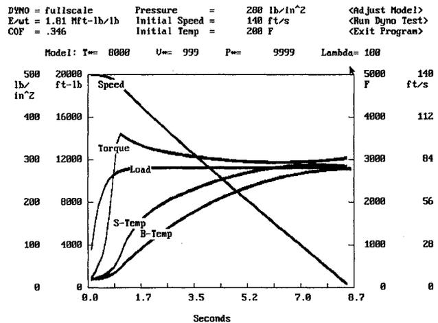
Figure 5. High energy stop for high thermal conductivity.
