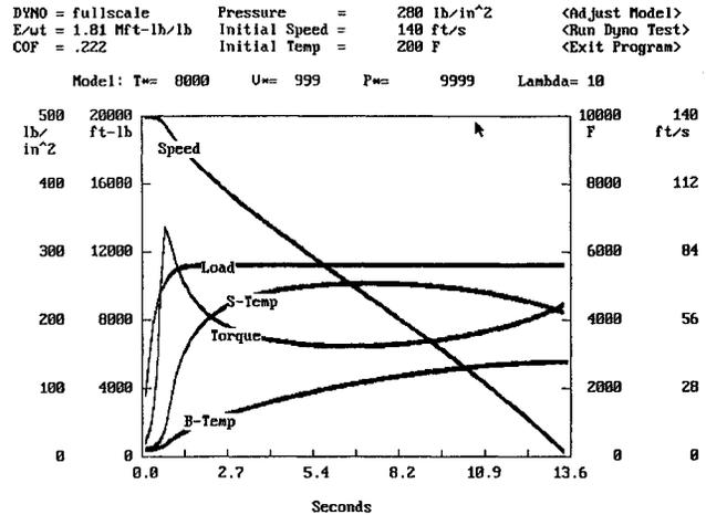
Figure 4. High energy stop for low thermal conductivity.
