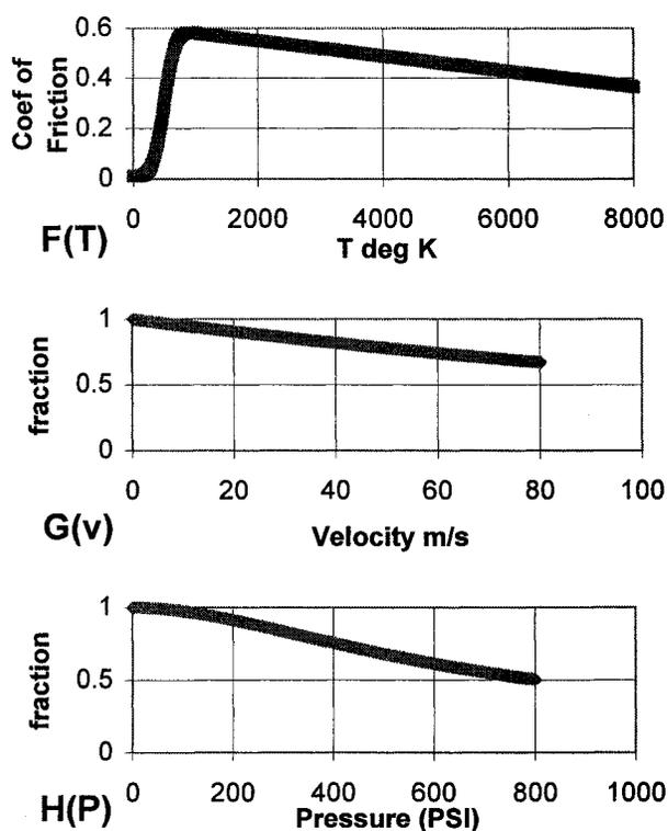
**Figures 1-3. Parametric friction model. One set of model parameters has been chosen resulting in the variations shown in these figures.**
