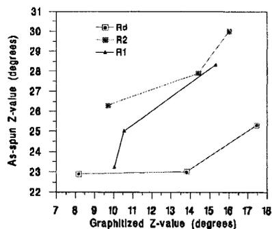
Figure 1. As-spun vs. Graphitized Z-value for R1, R2 and Rd.
