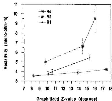
Figure 3. Electrical resistivity vs. Graphitized Z-value for R1, R2 and Rd (Based on 95% confidence interval).
