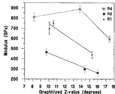
Figure 2. Modulus vs. Graphitized Z-value for R1, R2 and Rd (Based on 95% confidence interval).
