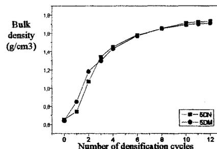
Figure 1. The bulk density variation of 5D C/C as function of number of densification cycles.
